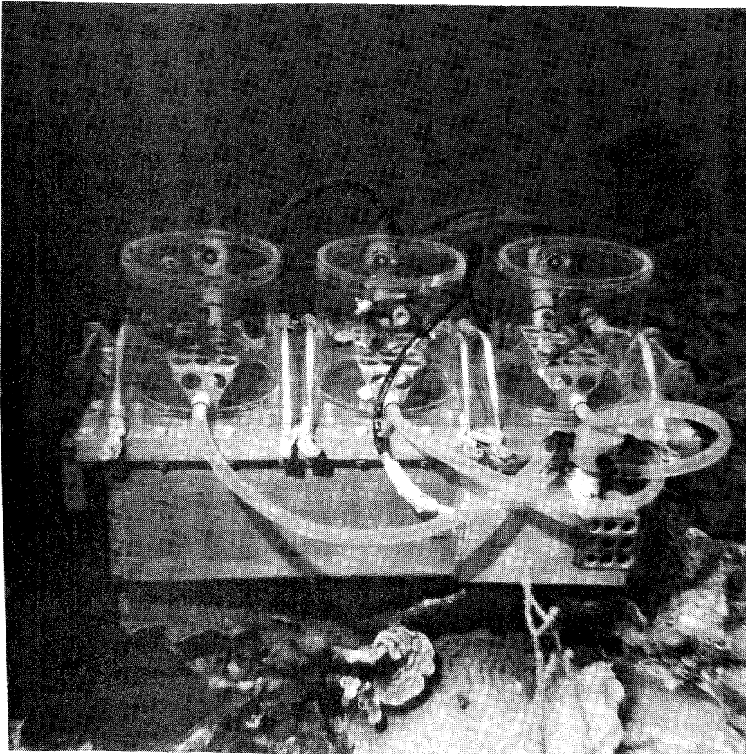
Fig. 1 The respirometer placed on corals at 20 m depth, in Virgin Island, St. Croix. It measures oxygen production from the zooxanthellz of the corals. (Photo: Dr. J. Porter)
