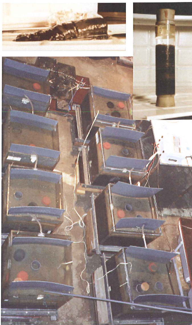
Figure 3. Set-up at Solbergstrand. Separate flows of oxic fjord water was added to the two boxes in front, flushing the sediments from the oxic location (left-hand row) and anoxic location (right-hand row) and the mussel aquaria in the back. The core (inserted) subsampled from the anoxic boxes divided along the laminae, almost like a stack of cards.
