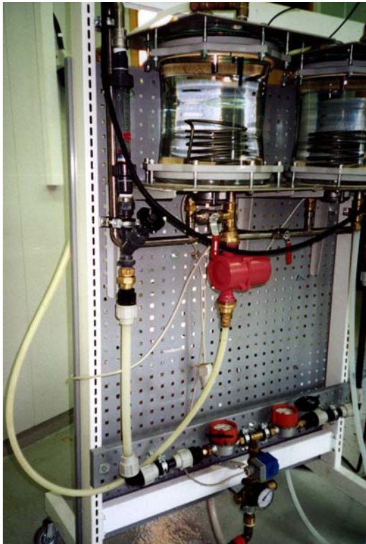
Figure 6: Left re-circulation loop without anti-scale device (front)
