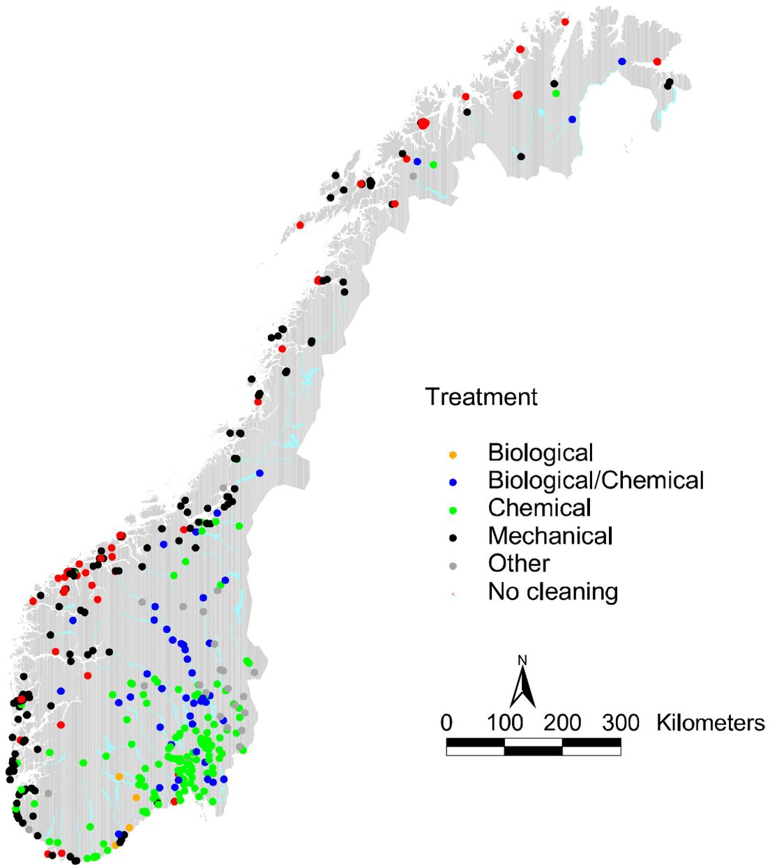
Figure 11. Treatment processes applied in wastewater treatment plants.
