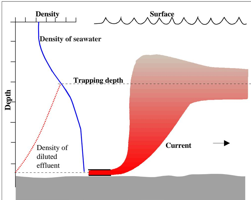
**Figure 19.** Example of deep water outfall with trapping of effluent below the surface.
