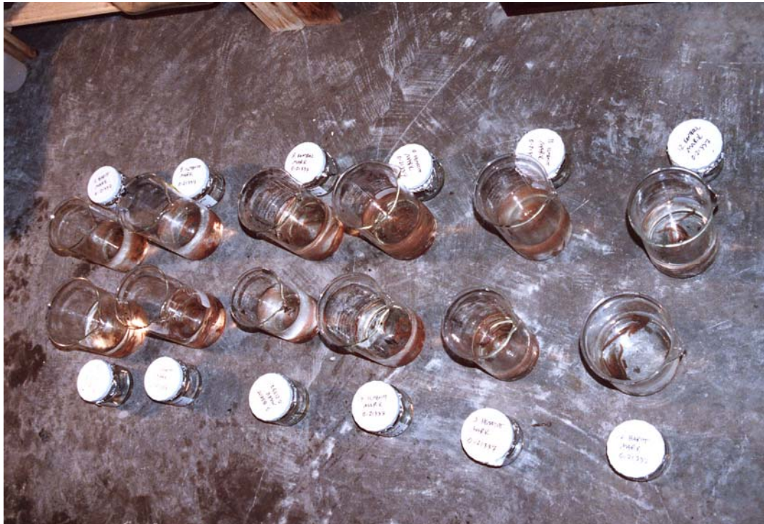
Figure 3. Ragworms, Nereis diversicolor (Polychaeta) held in beakers of seawater to empty the intestine from sediment residues.
