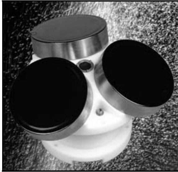
Figure 4. Photo showing the 3-beam transducer head on a NORTEK Continental ADP, which is a new version of the ADP used at Mongstad. The shape is quite similar for the old and new version. (The picture is from NORTEK's home page.)
