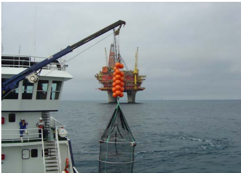
Figure 4. Deployment of cage containing fish and mussels, note the orange primary buoyancy elements.
