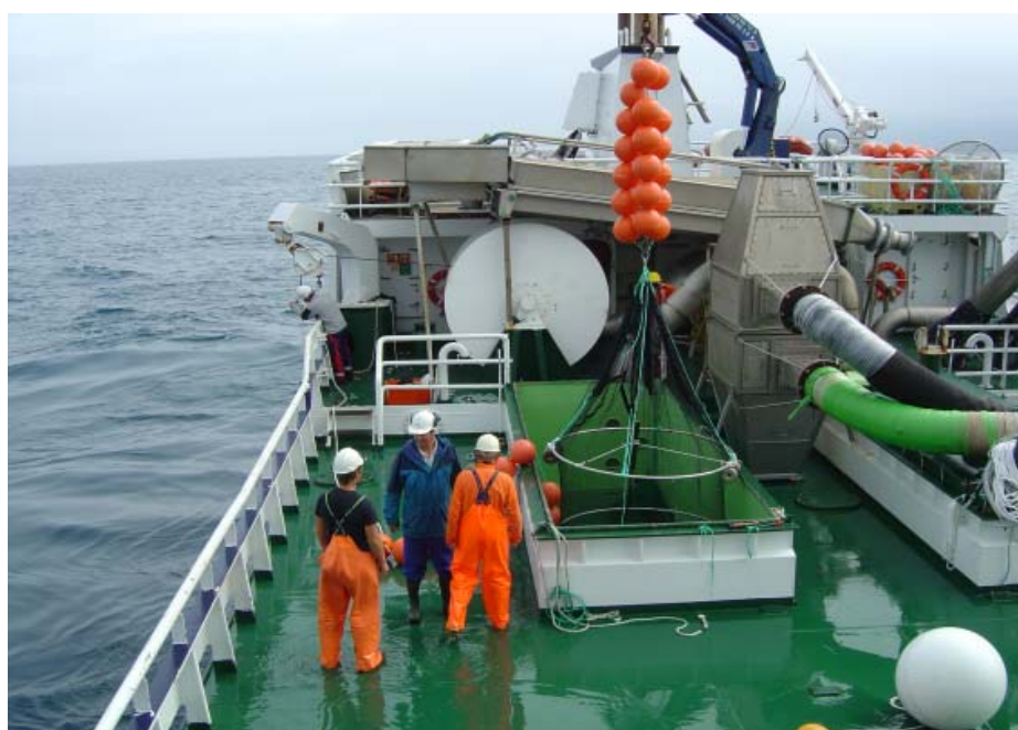
Figure 3. Preparation of cage with fish, mussels and SPMDs prior to deployment.
