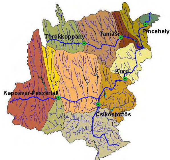
Figure 3.2. The figure shows the division of sub-basins and the monitoring stations used in the source apportionment calculation.
