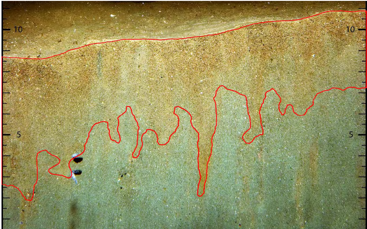
Measurement of aRPD. Enclosed aRPD (red area) is 77 cm 2 and mean depth of aRPD is 4.5 cm. (BHQ; aRPD = 4)
