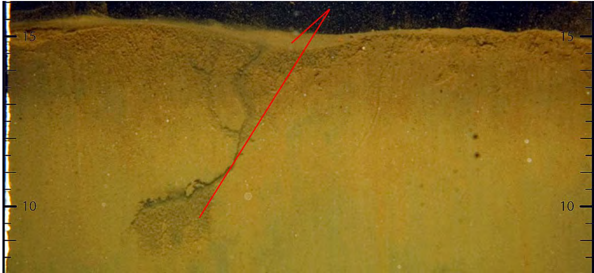
Pit with associated 'oxic void' connected to the sediment surface. Feature larger than 2 cm. The feature will not score for oxic void (BHQ; Pit or mound = 2)
