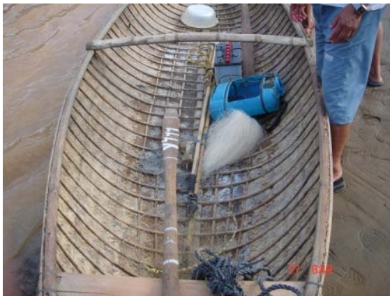
Bamboo boat equipped both with a gillnet and electric fishing gear.
