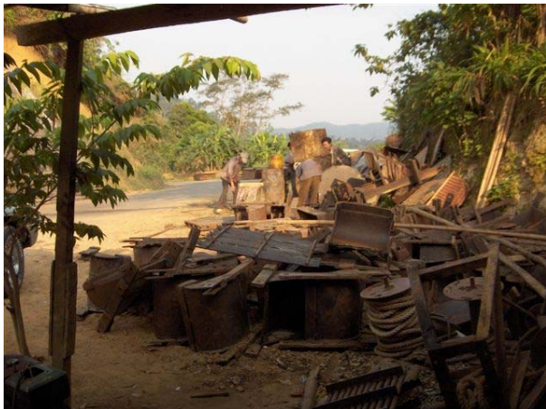
13. The dredging machines are pre-built in sections at small workshops in the forest.
