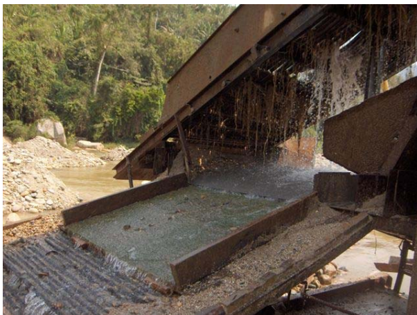
7. The gold and some sand are retained between the fibres in a nylon carpet, like the door mats used to clean dirty shoes.
