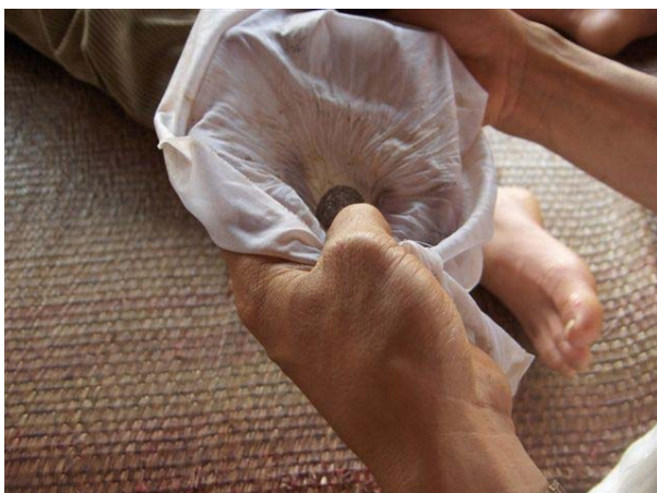
9. After a last mechanical separation where some coarse sand and debris are taken out, the remaining material is mixed with mercury and moulded in a cloth. The mercury reacts with the gold forming amalgam, the sand does not react. The surplus of mercury is squeezed through the cloth and collected.
