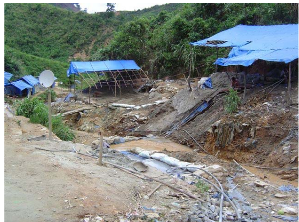
4. The water that escapes the rib settling system is led through ponds where more material settles out. The sediments here are taken up and led over the rib canal system once more for collecting more material.
