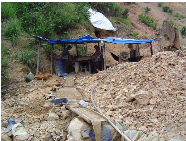
3. The crushed material is mixed with water, forming a slurry, which is led down a gentle sloping canal with a transverse rib system in the bottom. Heavy particles are retained between the ribs, while the lighter particles follow the water. The rib system is cleared for gold bearing particles at certain intervals.
