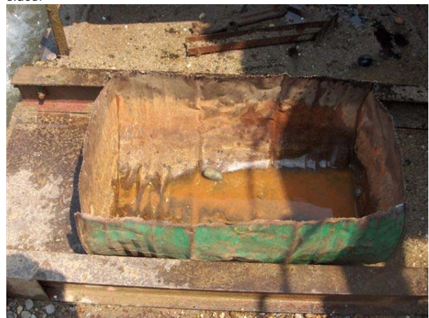
8. After some hours of operation the mats are thoroughly washed in a half barrel filled with water. The water is thereafter carefully decanted off.
