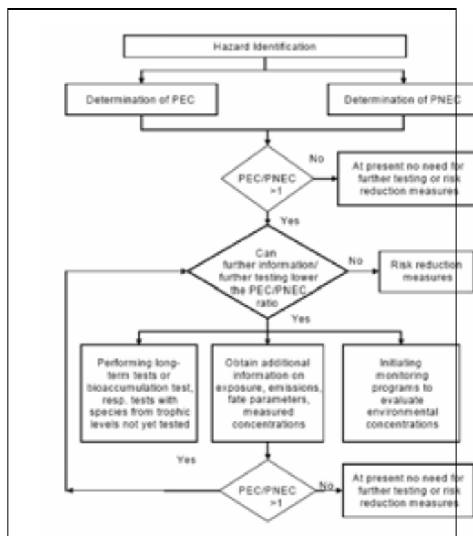
Figure 2 General procedure for environmental risk assessment according to the EU TGD
