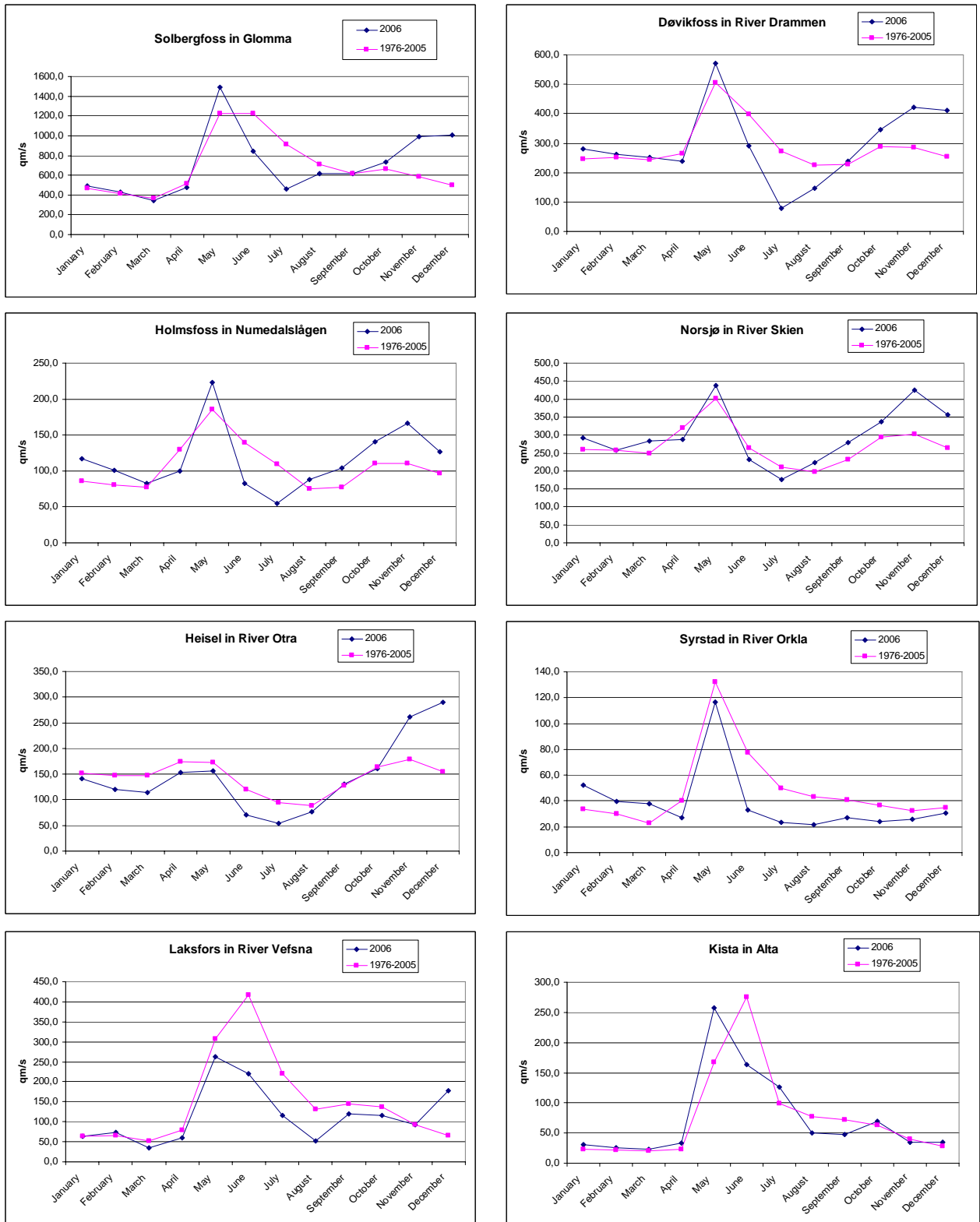
Figure 12. Monthly mean water discharge in 2006 and as an average of 30 years, derived from hydrological stations (named) in 8 of the rivers monitored monthly (data from NVE).
