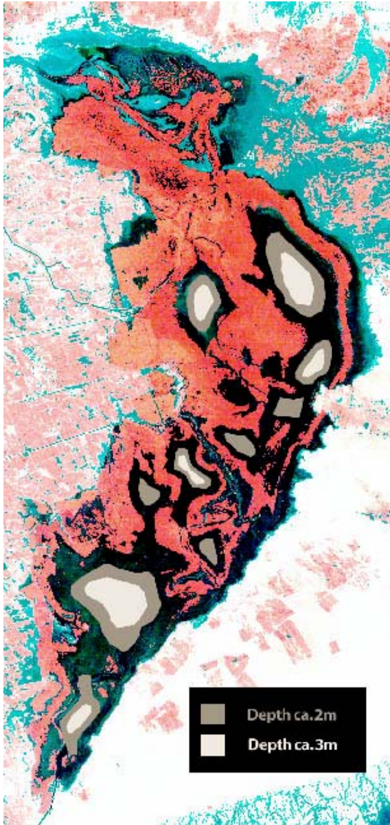
Figure 4.7 Example of how dredging of some areas could add to the increase in habitat diversity and, hence, the biodiversity of the lake. Construction of islands and peninsulas are other examples illustrating the same principles.
