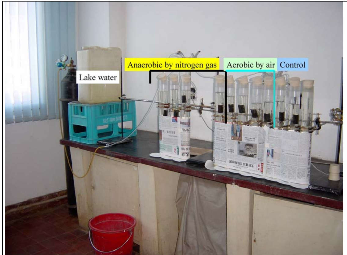
Figure 3.2 Sediment exchange experiment set up April 2002 at IMESI in Hohehot. Photo: Jonas Fejes
