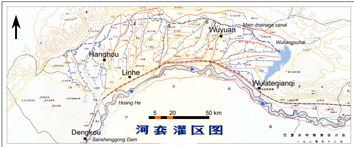
Figure 2: Map over Hetao Irrigation Area. Red lines are irrigation canals and blue dashed lines are drainage canals. Yellow lines are roads and black dashed lines are administrative borders. Along the main drainage canal at the northern border of the area are the numbers of the major drainage canals noted (Bayannaocer City Hydrological Bureau, 1980).
