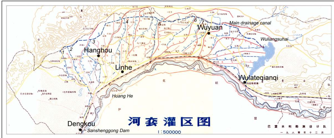
Figure 29. Map over Hetao and the irrigation system. Red lines are irrigation canals and blue dashed lines are drainage canals. Yellow lines are roads and black dashed lines are administrative borders. Along the main drainage canal at the northern border of the area are the numbers of the major drainage canals noted (BaMeng Hydrological Bureau, 1980).
