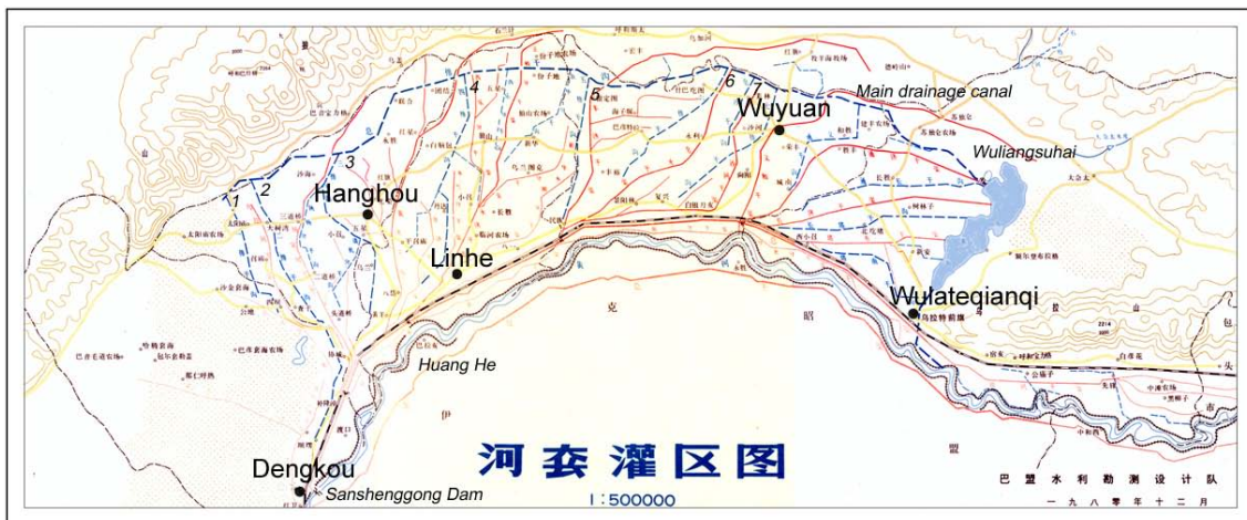
Figure 1. Map over the Great Bend of Yellow River with Hetao and the irrigation system. Red lines are irrigation canals and blue dashed lines are drainage canals. Yellow lines are roads and black dashed lines are administrative borders. Along the main drainage canal at the northern border of the area are the numbers of the major drainage canals noted (BaMeng Hydrological Bureau, 1980).
