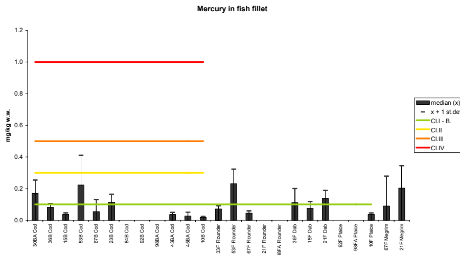
Figure 29. Median, standard deviation and upper limit to SFT Classes or provisional "high background" concentration for mercury in fish fillet 1990-1996 (A), 2006 (B) and 2007 (C), ppm (mg/kg) wet weight, "CI. – B" indicates that only upper limit to SFT Classes or provisional high background concentration is indicated for flatfish, (see maps in Appendix G).
