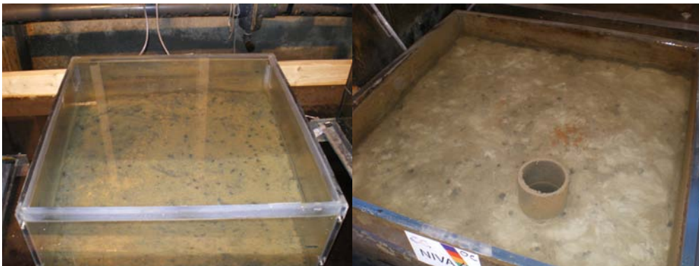
Figure 12. Sand (left) and olivine (right) caps 3 months after cap placement. Note: sediment layer integrity is preserved with the use of a tube placed following coring (right)
