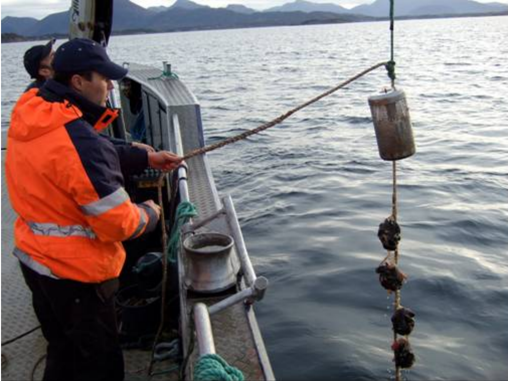
Figure 3. Retrieval of the mussels and SPMDs after 6 weeks exposure.
