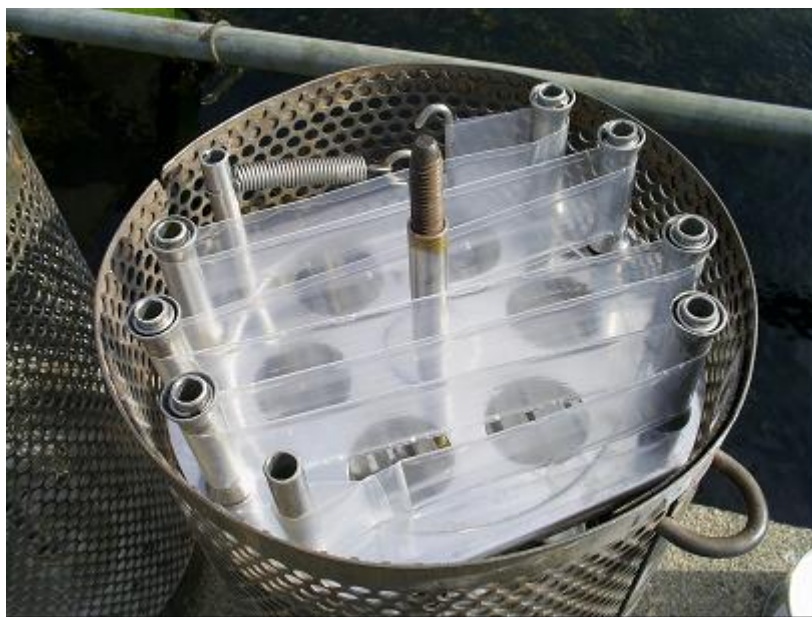
Figure 6. SPMD ready for use, mounted on a stainless steel spider in a deployment cage. (Photo source: Christopher Harman).
