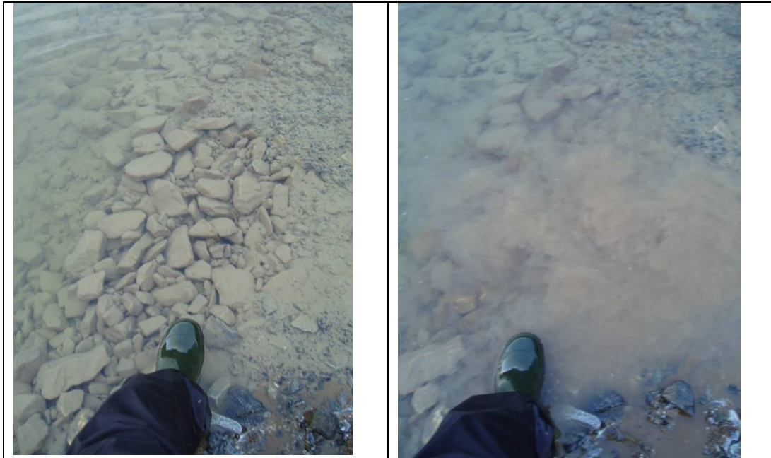
Figure 8. Fluffy, grey precipitates in lower dam at M17 before (left) and after careful disturbance of the limestone gravel.
