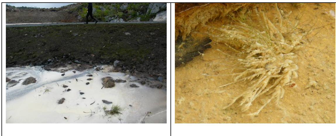
Figure 7. White precipitate at the dam barrier of M17, and attached to submerged plants and stream bed about 200 m downstream (May 18, 2009).
