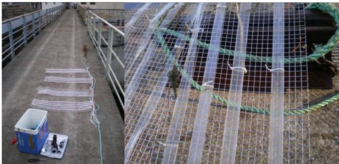
Figure 2. Passive sampler deployment setup using flat stainless steel cages to maximise turbulences around the samplers (left) and cages two weeks later with very little or in-existent biofouling. All samplers suffered significantly.
