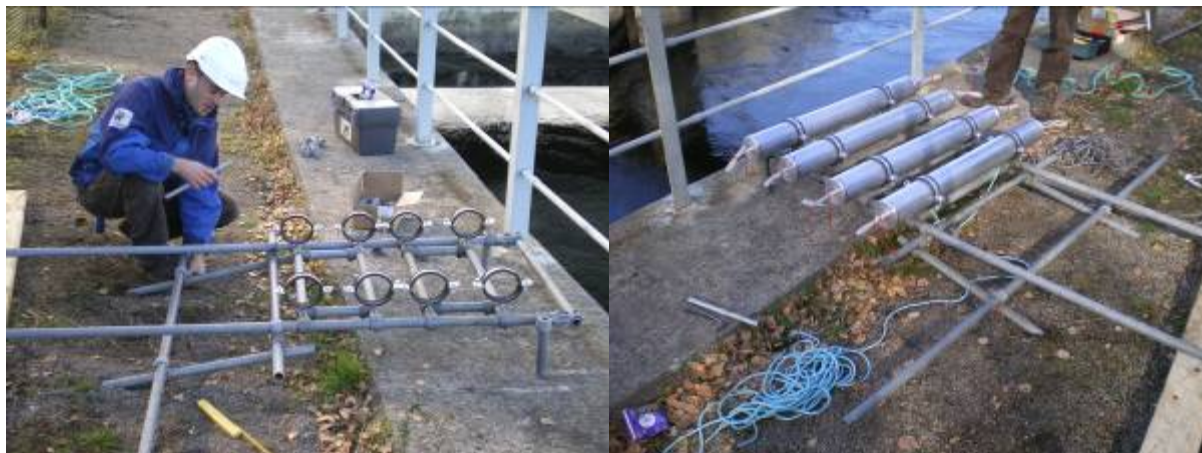
Figure 3. Frame for the deployment of the time-integrative SPM sampler (left) and 4 SPM samplers ready for deployment (right).
