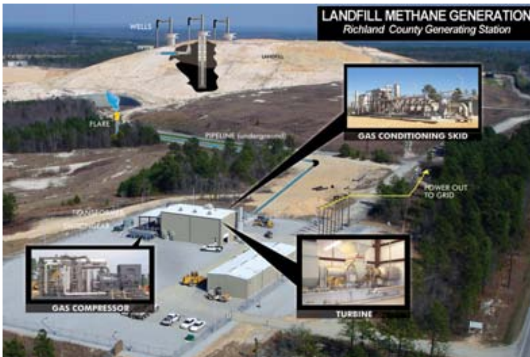
Figure 37. Landfill gas recovery http://www.scgreenpower.com/portal/page/portal/SCGreenpower/Images-Flash/gp_process.jpg
