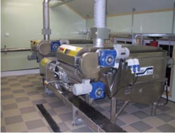
Figure 7. Salsnes filter developed by Salsnes Filter Company in Norway http://www.innovasjon Norge.no/TP_fs/Design/107-0730_IMG.JPG
