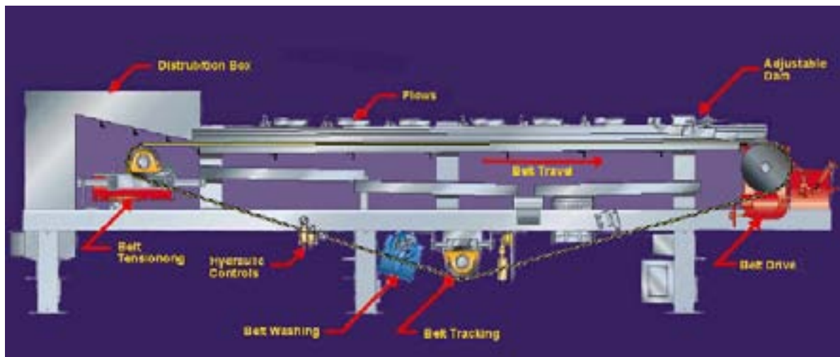
Figure 20. Belt thickener ( http://www.princeton-indiana.com/wastewater/Media/wastewater/biosolids/gravity-belt-thickner-2.jpg )
