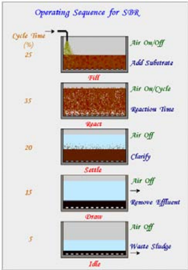
Figure 12. The principle of sequence batch processes for biological treatment ( http://www.enviroenergysystems.co.in/images/sbr1.jpg )
