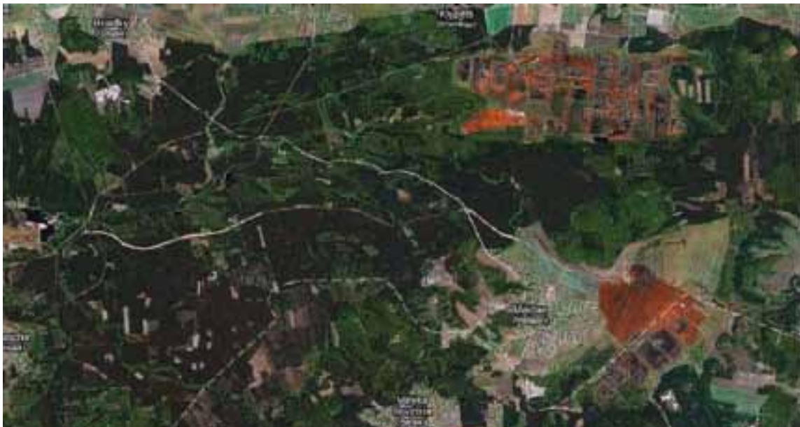
Figure 10. The right tributaries coming in from the east just upstream Dubno are considerably physically changed due to drainage and peat extraction (brown areas in the aerial photo).
