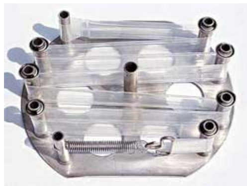
Figure 9. SPMD sampler correctly mounted on the holder
