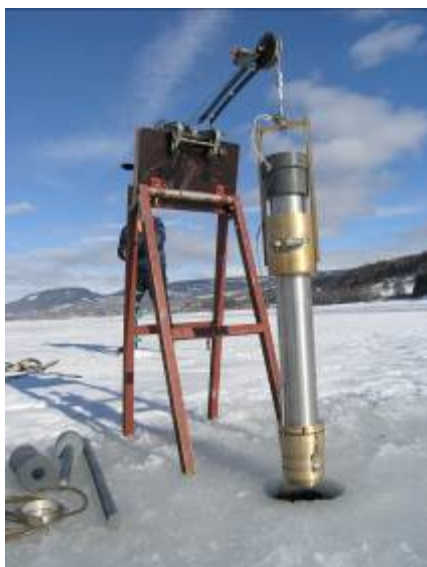
Figure 11. A gravity corer for layered sediment samples
