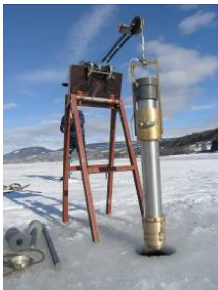
Figure 6. A gravity corer for layered sediment samples
