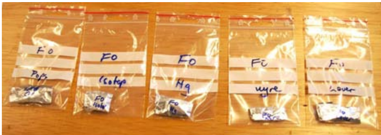
Figure 23. Tissue samples (muscle for POPs, Isotopes and Hg, kidney and liver) wrapped in Al-foil and placed in plastic zip bags. Both Al-foil and plastic bag must be marked with Fish code and type of sample.
