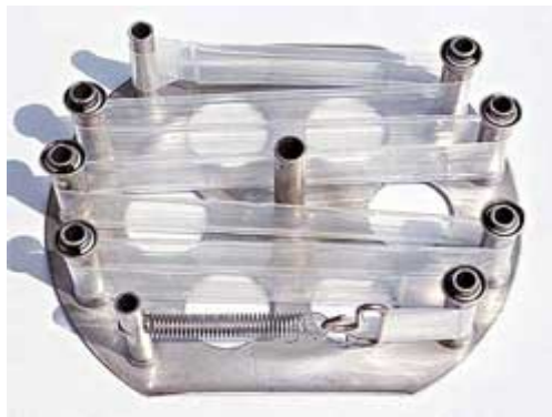
Figure 9. SPMD sampler correctly mounted on the holder
