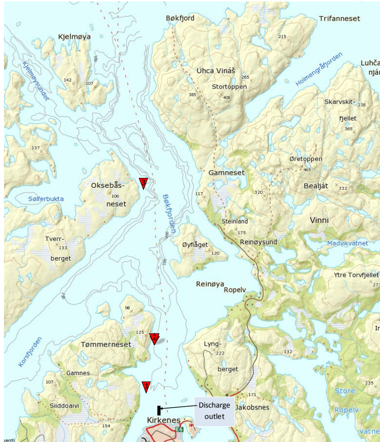
Figure 1. Approximate locations of the three field mussel groups in Bøkfjorden in relation to the Sydvaranger mine discharge outlet. Approximate distances from the outlet: group 1 – 0.6 km; group 2 – 3 km; group 3 – 10 km. Group 4 – From Brashamn 40 km (source of the mussels, not on the map).
