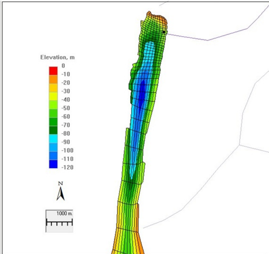
Figure 12. The grid was more detailed (finer spatial resolution) near the power plant outlet.
