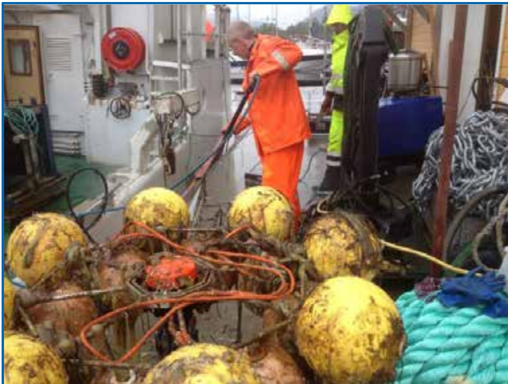
Figure 4. Top of the current meter gimball frame after recovery in May, 2013.
