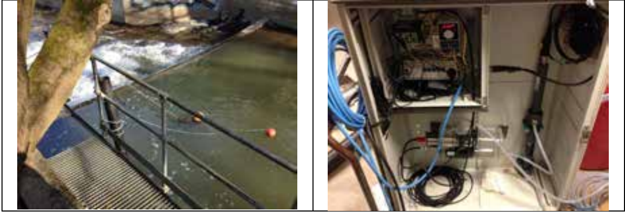
Figure 2. Continuous monitoring of pH, conductivity, turbidity and temperature in a RID river (photo: NIVA).
