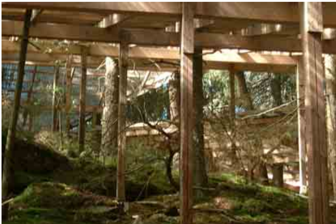
A plastic roof was constructed over the catchment G1 at Gårdsjön, Sweden in 1991.
