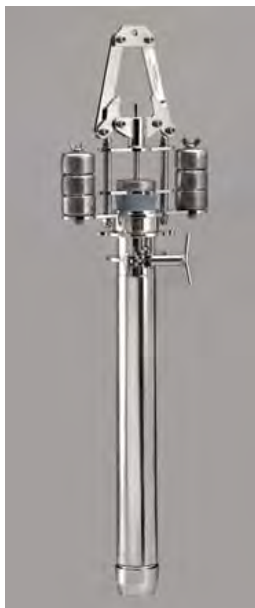
Figure 8: Kajak corer: 5.5 cm in diameter.
