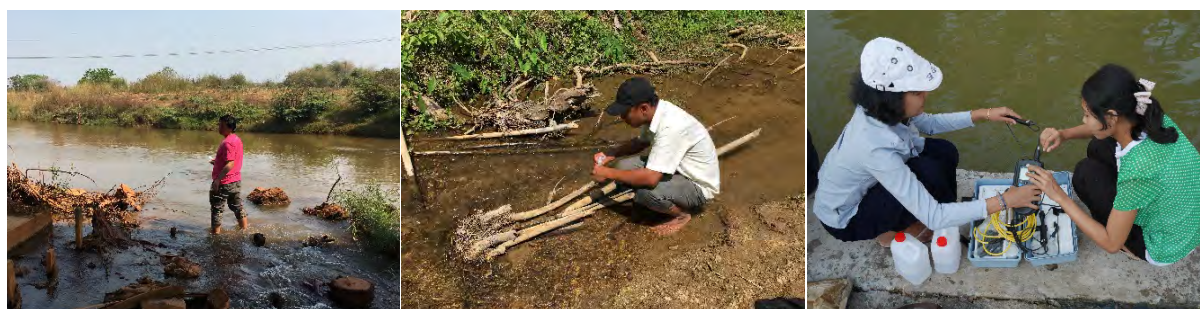
Figure 4.3. Water chemistry sampling in a bottle (left and center) and with a oxygen probe and pH-meter (right).
