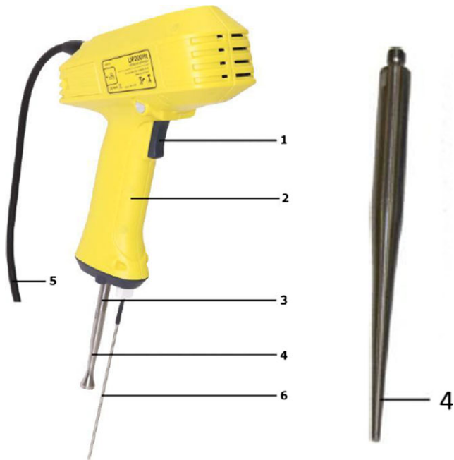
FIGURE 1 Left: Ultrasonic Processor UP200Ht from Hielscher. 1-activation trigger, 2-handhold, 3-sonotrode attachment, 4-sonotrode, 5-power cord, 6-temperature probe. Right: The Sonotrode used in the experiments (S26d2, 2 mm). Photos: Hielscher, Germany, ©www.hielscher.com, 2016 [Colour figure can be viewed at wileyonlinelibrary.com]
