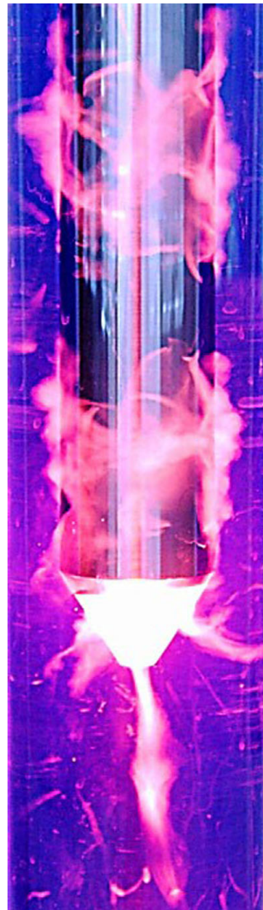
FIGURE 2 Example image of cavitation around Sonotrode. Photo: Hielscher, Germany, ©www.hielscher.com, 2016 [Colour figure can be viewed at wileyonlinelibrary.com]
