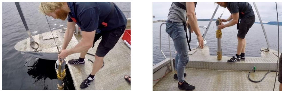
Figure 2. Deployment of Kajak-Brinkhurst sediment corer during sampling in Lake Mjøsa and Lake Femunden. Images show core being deployed (A) and retrieved (B) at the stern of the vessel. Images: David P. Eidsvoll, NIVA.
