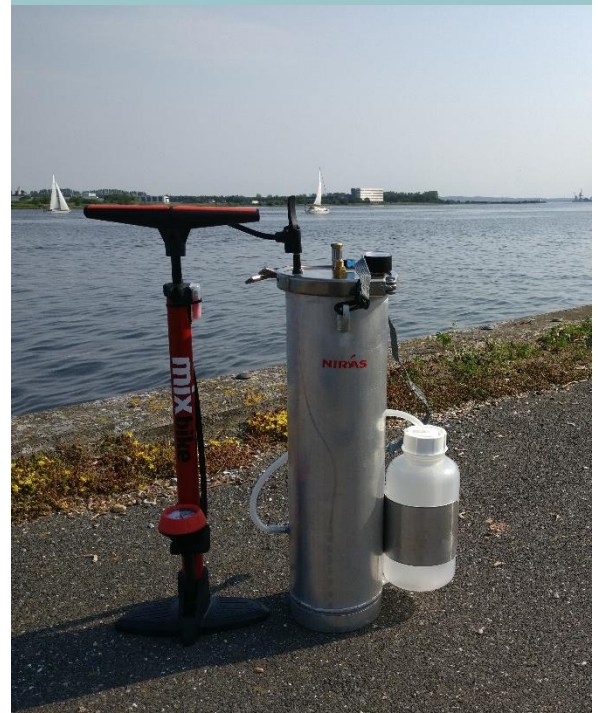
Add pressure to start filtration
