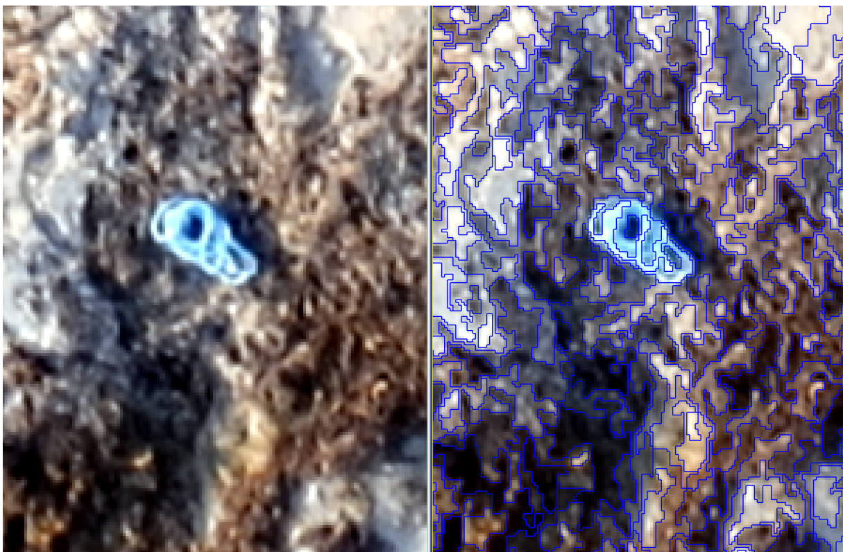
Figure 17. Screenshot from the eCognition essentials software package with an example of a blue plastic piece (a rope) and the segmentation depicted as polygons with blue outlines. The right picture shows the plastic object divided into several segments, termed over-segmentation. The example originates from the RGB orthomosaic from Akerøya (scenario 1).
