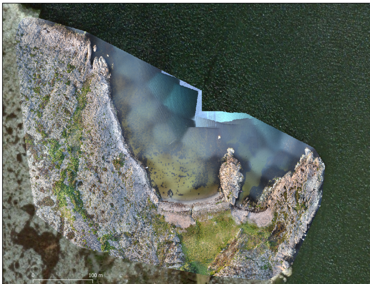
Figure 10. An RGB orthomosaic of Akerøya 2019 captured from 55 m altitude, with a 1.6 x 1.6 cm pixel resolution of the ground. Satellite imagery is used as background (Google Earth).
