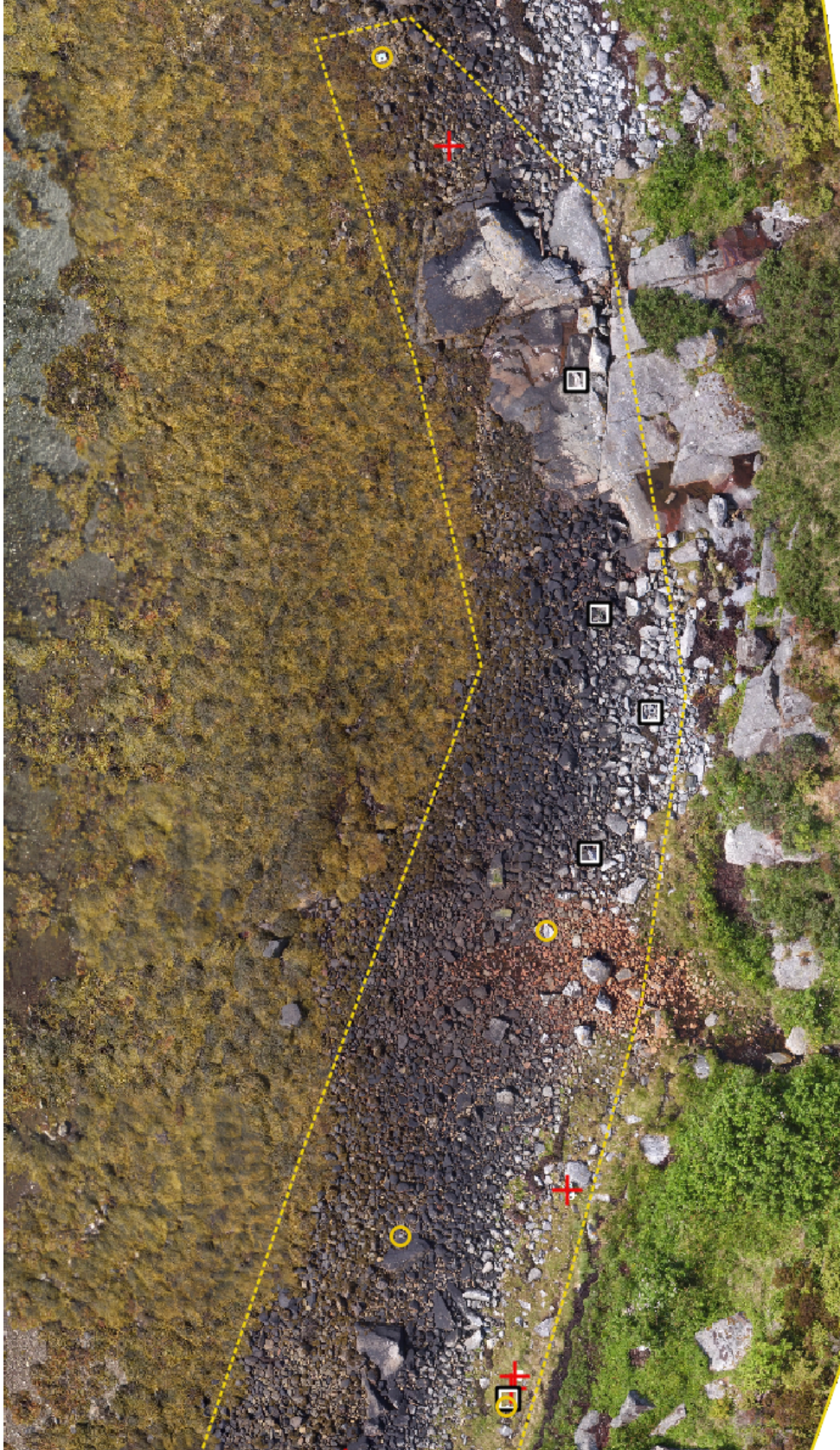
Figure 27. Scenario 3 northern half: Location of detected plastic pieces are marked with red crosses; non-detected pieces are marked with black squares. Plastic pieces used for training data are marked with yellow circles.
