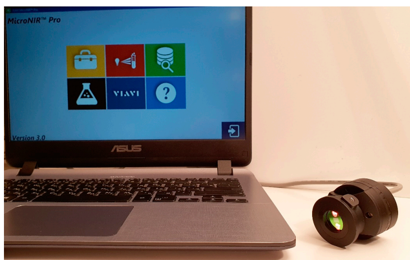
Figure 1. Ultra-compact near infrared (NIR) spectrometer MicroNIR 1700ES.
