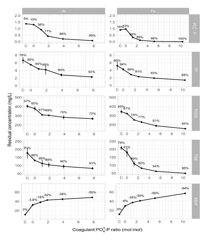
Figure 1: Effect of different molar doses of FeCl<sub>3</sub> (right-side figures) and AlSO<sub>4</sub> (left-side figures) on the removal of PO<sub>4</sub><sup>3</sup>-P, TP, TSS and production of sludge, expressed as SSV<sub>f</sub>, in the sludge flow stream using
