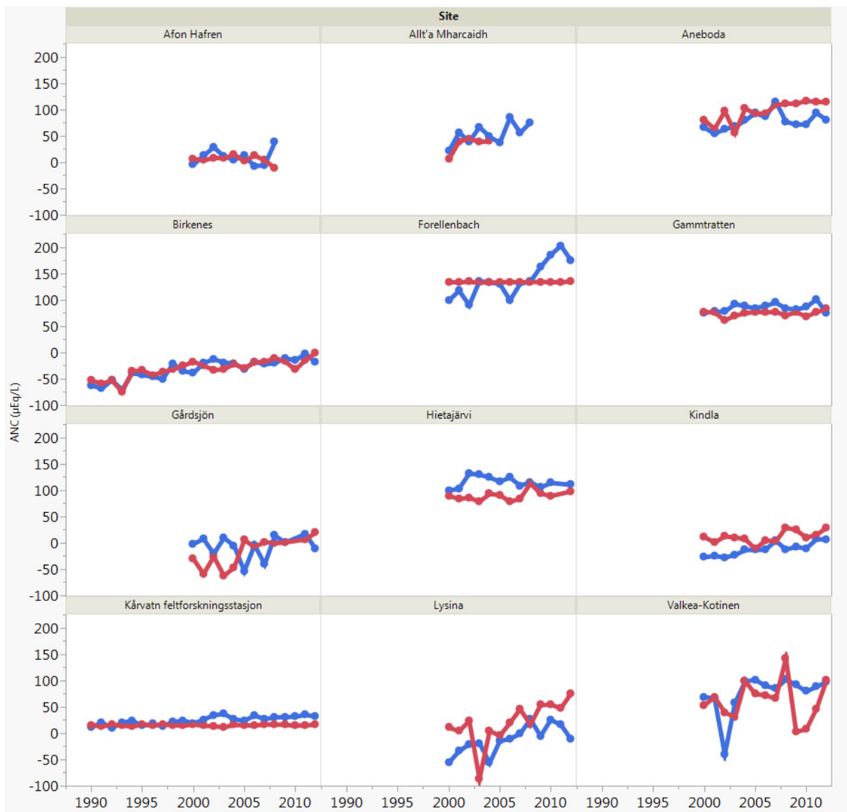
Figure 20. Annual average measured (blue) and estimated (red) ANC in surface waters at 12 ICP IM stations.
