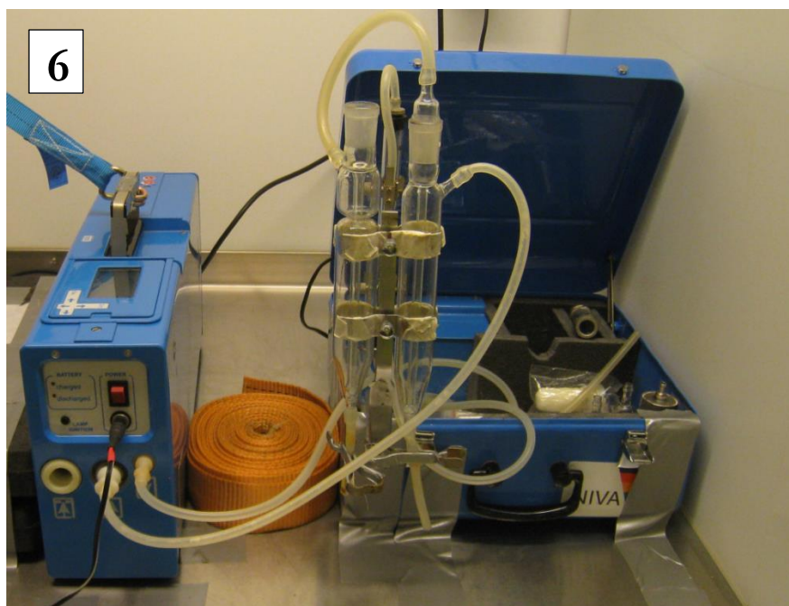
Picture 6. Water samples were analysed with a portable Lumex Zeeman Mercury Analyzer RA-915+, with a RP-91 attachment (photo: Sigurd Øxnevad, NIVA).
