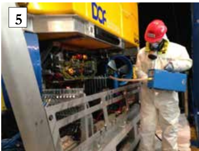
Picture 5. Measurement of mercury in air around a ROV that had just been landed on deck (photo: Phillip Andersen, Franzefoss).
