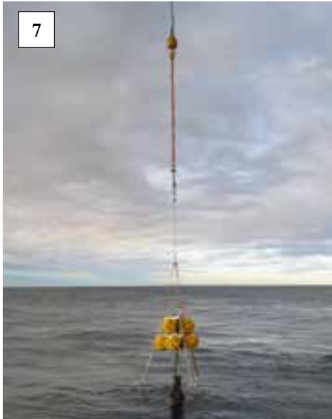
Picture 7. Tripod with water current profiler and turbidity sensor being deployed (photo: Sigurd Øxnevad, NIVA).
