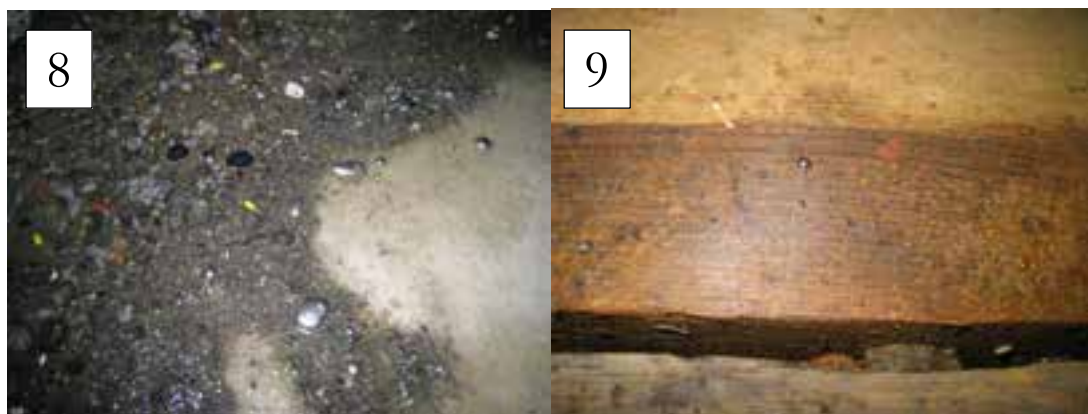
Pictures 8 and 9. Mercury and sediment on the silt cloth (8), and mercury on the wooden deck (9) (photos: Sigurd Øxnevad, NIVA).
