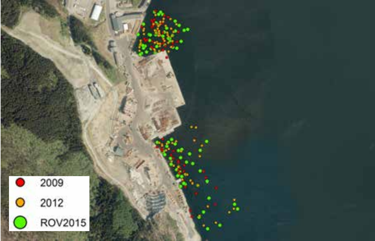
Figure 7: This overview picture shows the positions of all anthropogenic materials that have been registered and positioned during the ROV surveys conducted in 2009, 2012 and 2015.
