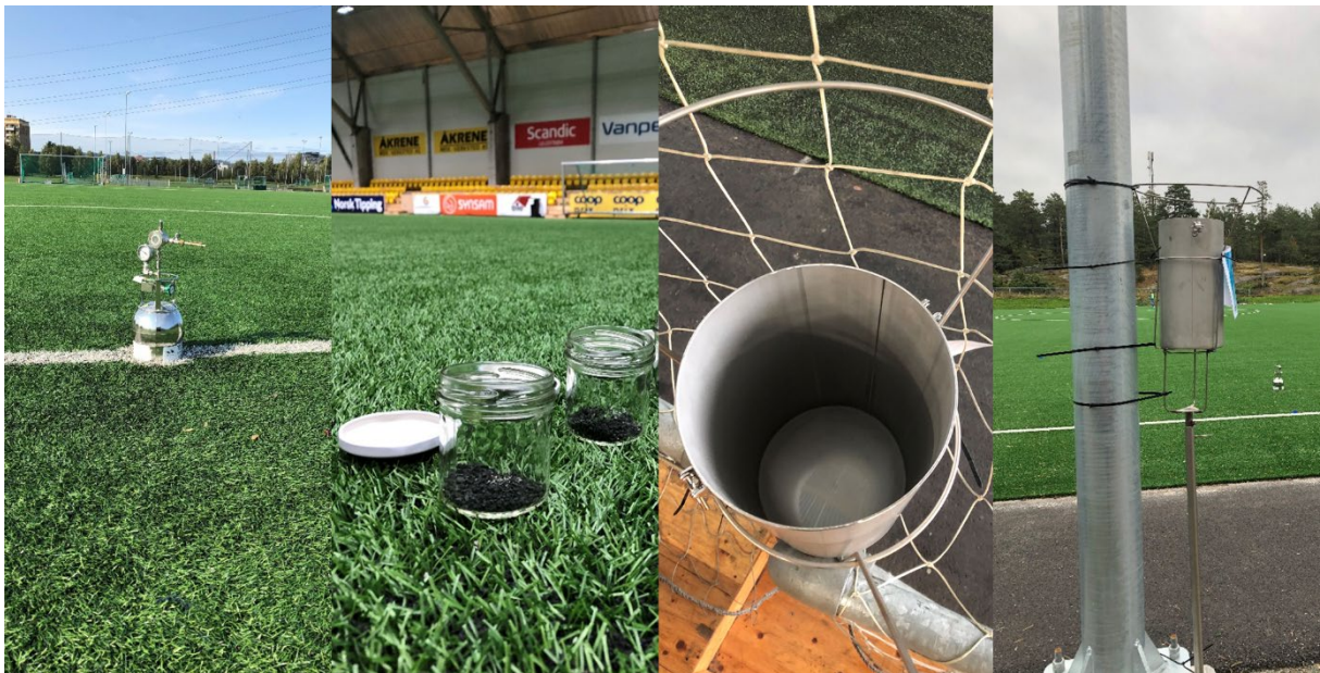
Figure 3: Sampling of air, granules and deposition of airborne plastic particles at artificial turfs. (Photo: Heidi Eikenes, Helene Lunder Halvorsen, Pernilla Bohlin-Nizzetto, NILU.)
