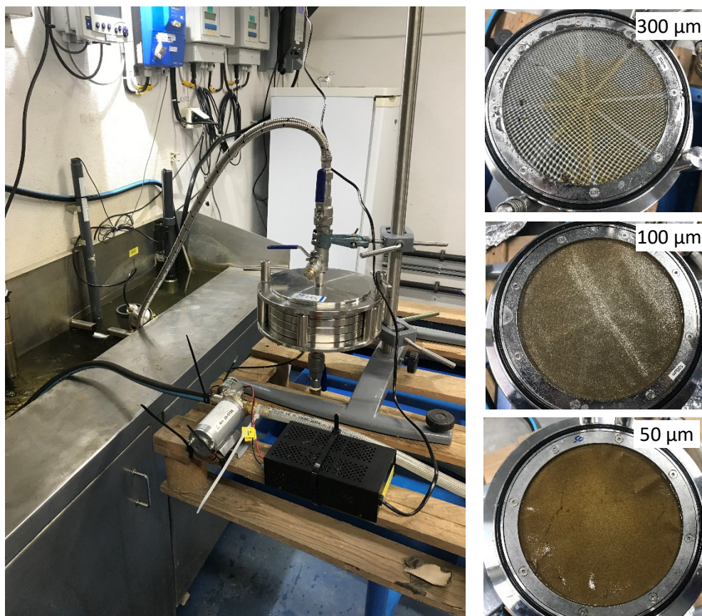
Figure 7: Setup for sampling microplastics in the effluent from Bekkelaget WWTP. The sieves to the right show the collected material after sampling on October 8 th 2020. (Photo: Christian Vogelsang, NIVA.)
