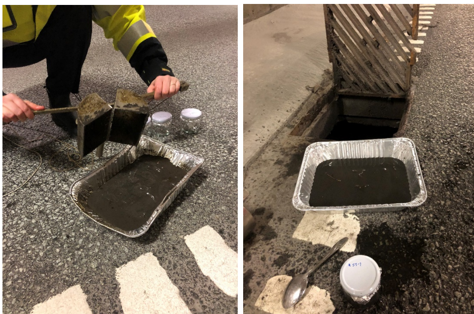
Figure 9: Sediment from gully-pots were collected using a small Van Veen sediment sampler. (Photo Elisabeth Rødland, NIVA.)
