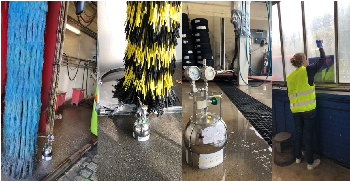
Figure 2: Sampling of air and surface dust at vehicle washing facilities. (Photo: Heidi Eikenes, Helene Lunder Halvorsen, Pernilla Bohlin-Nizzetto, NILU.)
