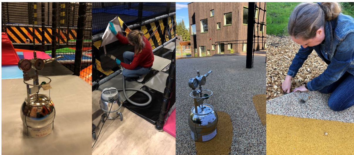
Figure 4: Sampling of air, settled dust and granule sampling on rubber flooring playgrounds. (Photo: Heidi Eikenes, Helene Lunder Halvorsen, Pernilla Bohlin-Nizzetto, NILU.)
