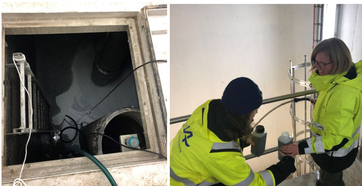
Figure 10: Sampling of tunnel wash water during a tunnel wash in the Smestad tunnel pump station. (Photo: Elisabeth Rødland/Sondre Meland, NIVA)
