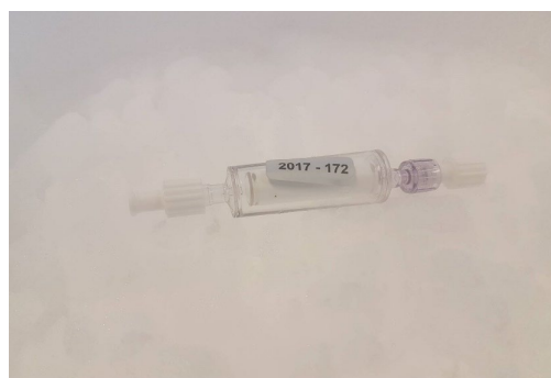
Figure 3.16: After carefully emptying all water the Sterivex filter is labelled with unique label, luer-lock stoppers attached and stored on dry ice.
