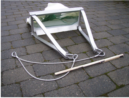
Figure 3.8: Hand-operated dredge (40 cm x 20 cm) for collecting sediment epifauna.
