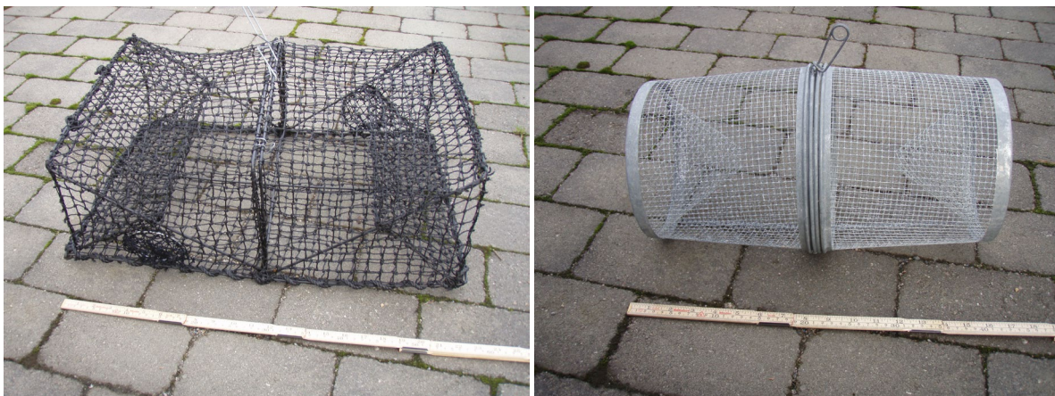
Figure 3.5: Crab trap (left) and Gees minnow trap (right) used for sampling of mobile epifauna in Aarhus and Esbjerg harbours.
