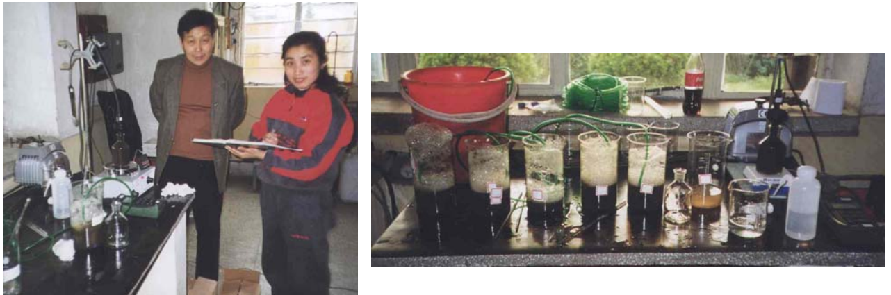
Figure 40. Biological Oxygen Uptake Rate tests of domestic waste water and industry waste water. Picture shows oxygen measurements in a test-bottle (left) and parallel aeration of test bottles (right).
