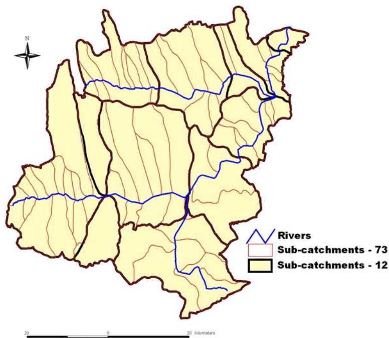
Figure 4.1. The delineation of the Kapos catchment into 12 (black lines) and 73 sub-catchments (brown lines).
