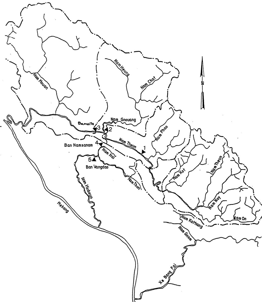
Figure 1. Overview of the area for the Nam Theun Hinboun Hydropower Project. 100 m 3 /s is going to be diverted from Nam Theun to Nam Hai.
