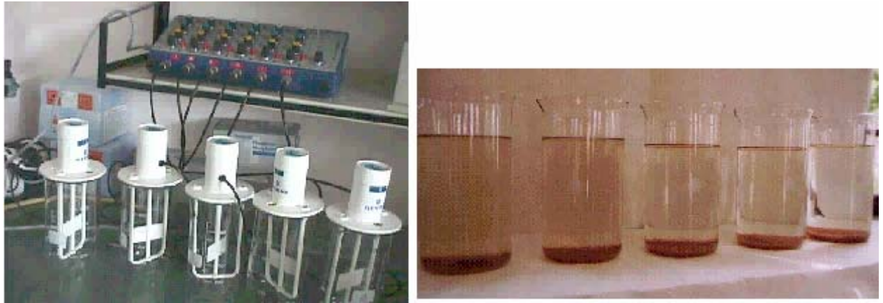
Figure 39. Automatic Jar-tests equipment, and jars after sedimentation.
