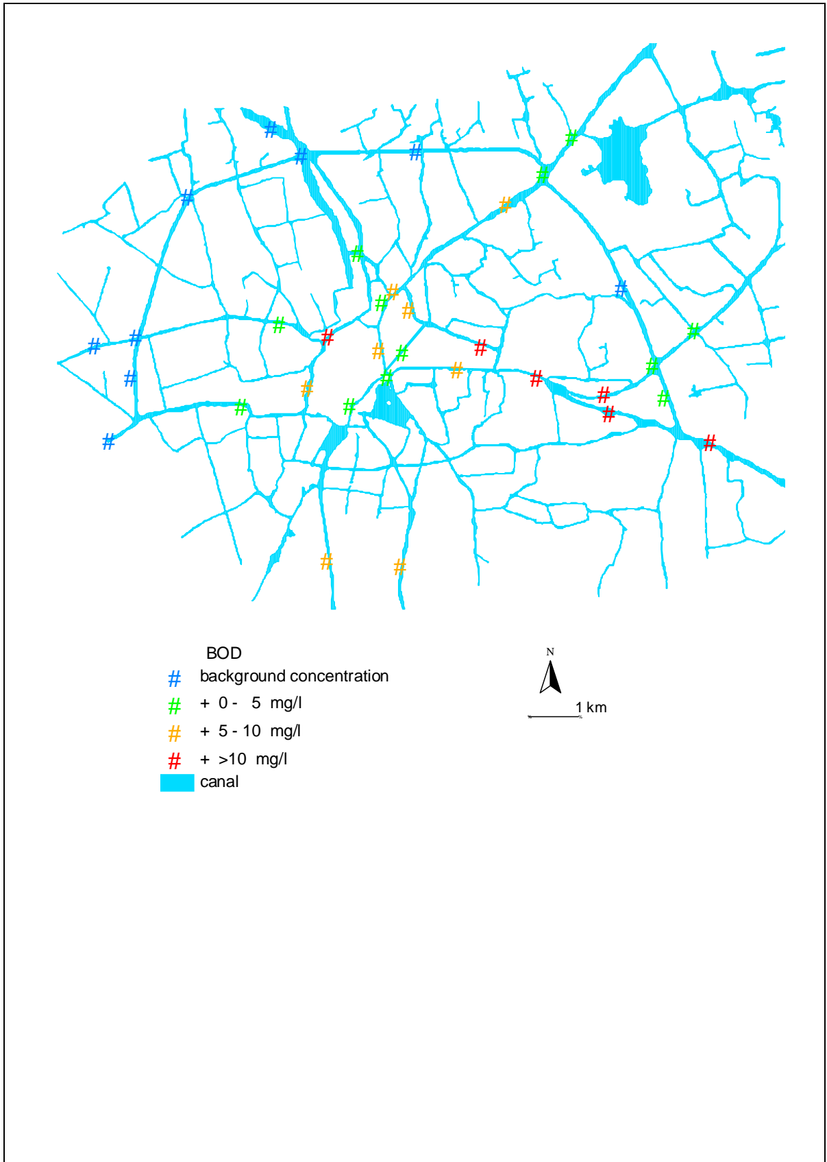
Figure 21: Increase in biological oxygen demand, BOD, above background concentration for the year 2020 at median water flow, no treatment plant.
